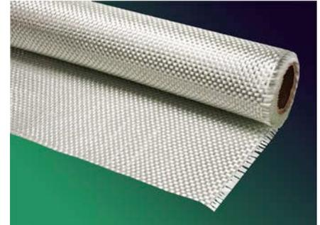
should not exceed 35 °C (95 °F) and the relative humidity should be kept below 75%. Fiberglass products must remain in packaging material until just prior to their use. If these conditions are respected, the glass fiber product should not undergo significant changes when stored for extended periods of time.
